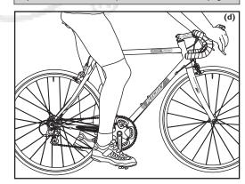
Take care not to over-tighten the clamping mechanism of the seat tube. Too strong a clamping force can cause the seat post and/or the frame to fail, which can lead to an accident and possible injury to the rider.
