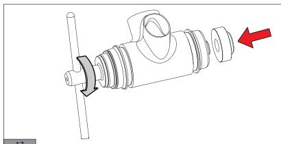
• Turn the lever of tool UT-BB140 clockwise until both bottom bracket cups are flush with the bottom bracket (Fig. 18).
