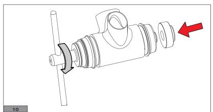
• Turn the lever of tool UT-BB140 clockwise until both bottom bracket cups are flush with the bottom bracket (Fig. 11).
