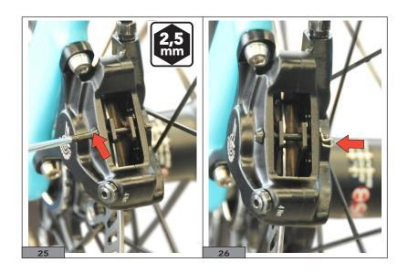
**25)** Align the calliper with the disc keeping the brake lever pressed and tighten the two calliper screws (Fig. 27).
