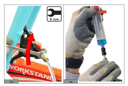
**13)** Check that there is oil in the screw seat and tighten the bleed screw (Fig.15).
