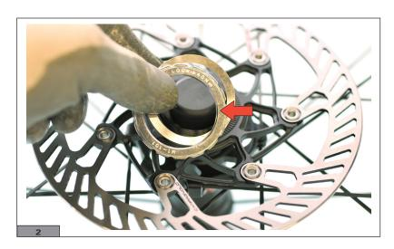
3) Screw on the locknut (Fig.3).
