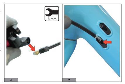
The barb driver on the end of the hose can be used to guide the hose via a rear derailleur hose mounted onto it (Fig.).
