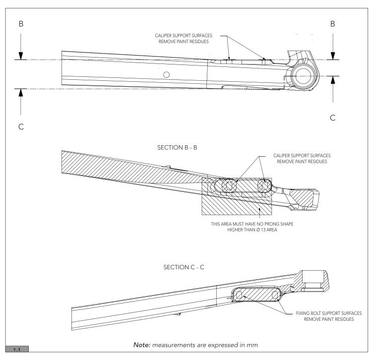
• Using the frame cutter tool make sure the calliper contact surface on the fork and the left-hand chain stay are perpendicular to the discs, grinding the chain stay if necessary in order to achieve this (Fig.2).
