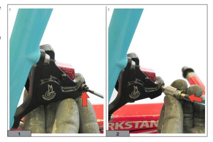
**3** Open the valve by turning the nut on the valve itself anticlockwise by approximately ¼ turn (Fig.3 - Fig. 4).
