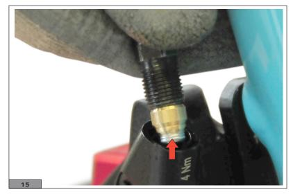
**16)** Insert the hose into the calliper once again, screw on and tighten the nut again to the prescribed torque, taking care not to damage the hose with the tool (Fig. 17).
