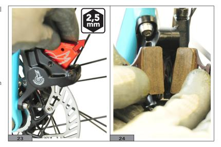
23) Mount and tighten the pad pivot (Fig. 25).
