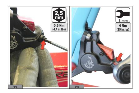
**19)** Using alcohol, clean away any oil from the calliper (Fig. 21).
