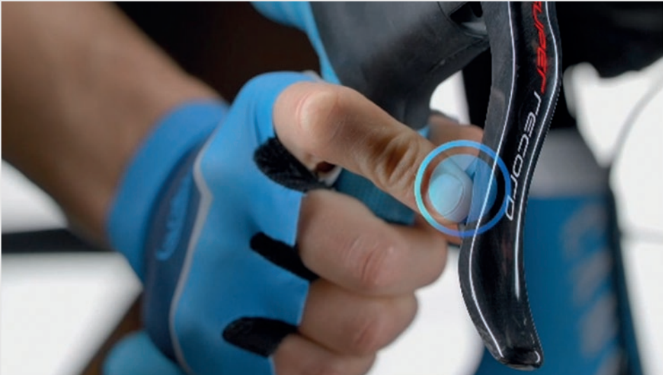
Upshifting lever incorporated into brake lever
