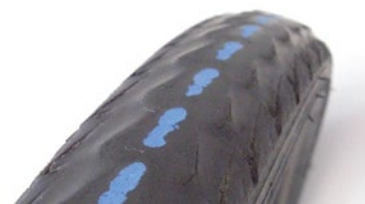
The puncture protection layer can be seen. The tire must be changed urgently.
