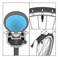
The correct fitting of the tire on the rim is mostly notable by a loud clicking noise. Check the air tightness of your Tubeless system. Does it lose any air? Check if the control line has an equal distance to the rim. If not release some air and work on the tire with both hands.
