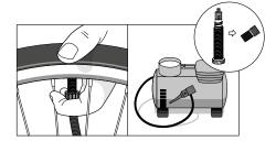
To fit the tire between the hooks, you may need a higher amount of air in the first instance. If you are using a floor pump, it is better to maintain a constant momentum within the first few seconds. A modern floor pump with a second inflatable cartridge can help to achieve this.
