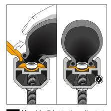
Mount the Tubeless tire on the rim in correct orientation of rotation. Ensure no loose pieces (e.g. sand, plastics) are found inside. Due to the tighter dimension tolerances of a Tubeless tire compared to a normal Clincher tire it may be helpful for you to use tire levers.
