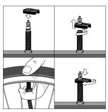
To enhance the air volume, unscrew the valve core. Pump it up and screw the valve core in again.
