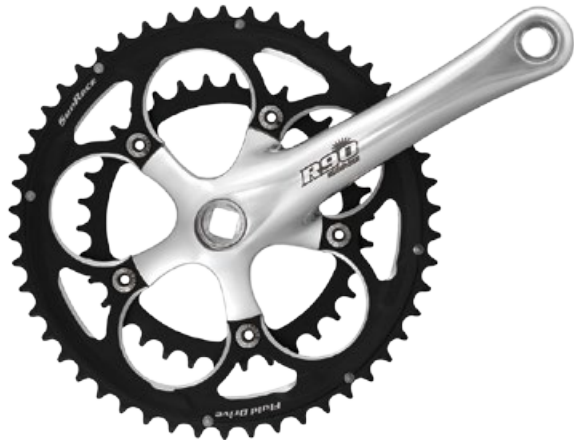
FCR9F 50-34T FCR9A 53-39T [9-Speed] [Alloy Chainrings] [SCM435 Bolts & Nuts] [6061 Forged Alloy Crank] 600g[9F] / 697g[9A]
