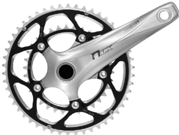
FCRX6 [D1] 50-34T FCRX1 [D1] 53-39T X7 [D1] 50-36T X3 [D1] 52-39T [BCD 110mm] [BCD 130mm] [10-Speed] [6061 Forged Alloy Crank] [Chromoly ISIS Axle] [7075 Chainrings] [7075 Bolts & Nuts] [7075 Axle Bolt] 944~956g [incl. BB]
