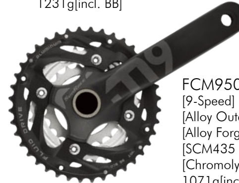
FCM958 48-36-26T [9-Speed] [Alloy Outer Chainring] [Alloy Forged Cranks] [SCM435 Bolts & Nuts] [Chromoly Axle] 1231g[incl. BB]
