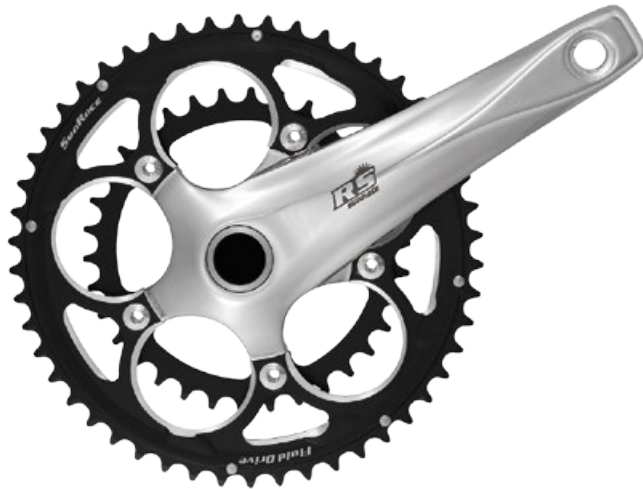
FCRS6 (S1) 50-34T FCRS1 (S1) 53-39T [BCD 110mm] [BCD 130mm] [10-Speed] [6061 Forged Alloy Crank] [Alloy Chainrings] [7075 Bolts & Nuts] [7075 Axle Bolt] 944~949g [incl.BB]
